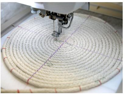
For best results, we will be floating the coil rather than trying to hoop it. Floating involves hooping the stabilizer firmly by itself. Then, the fabric (or coil in this example) is glued onto the stabilizer with temporary spray adhesive. Hand sewn stitches are used around the edge for extra security and will be shown in a later step.
