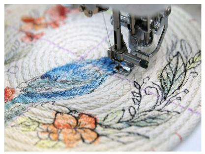
Attach the hoop onto the embroidery machine and center the needle over the center of the drawn lines. Load the embroidery file. For this project, we recommend using a 75/11 sharp sewing needle. This type of needle has a finer point and will make smaller perforations in the stabilizer and rope. Follow the color change sheet and embroider the entire design.
